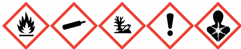
Flammable Compressed Gas Environmental Hazard Irritant Health Hazard
